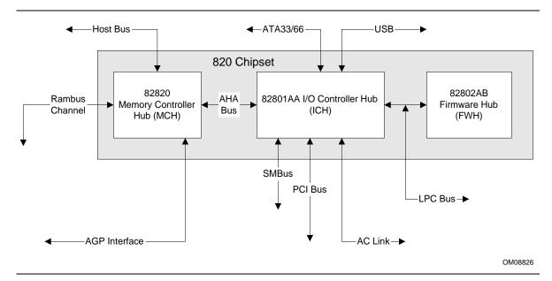
Figure 3. Intel 820 Chipset Block Diagram
